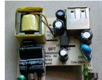
Part No: GAD050502 Adapter, input: 100~240Vac, output: 5V/1A
