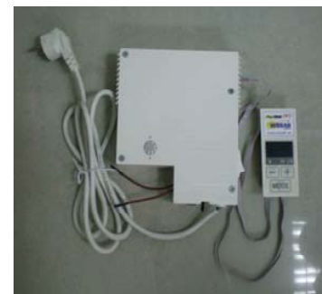
Part No : DIGI Thermostats, input: 230Vac, output: 230Vac/2000WMax
